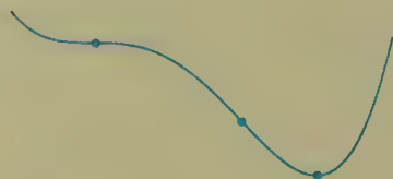
Figure 5.31 The graph for f has no extremum but has points of inflection where x = 0 and x = 2 , and a local minimum where x = 3 . (Example 7)
